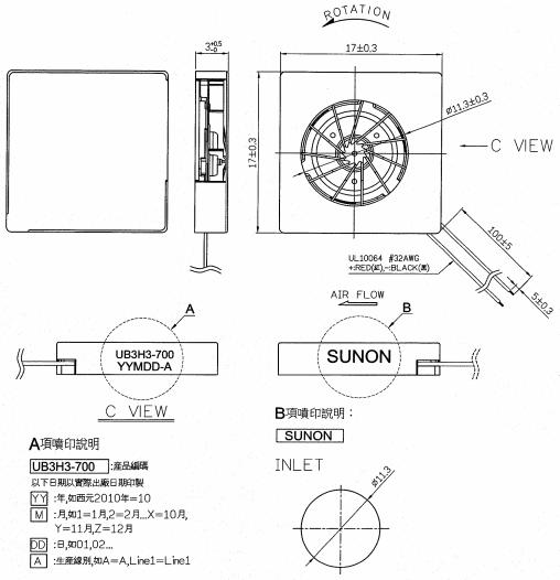
Sunon standard sample exclude the connector. If there is any request for connector, please advise in advance. About recommend connector, SUNON recommend the following models for SUNON Mighty Mini Fan/Blower: 1.(JST) SUR series connector: 02SUR-32S / 03SUR-32S / 04SUR-32S.
