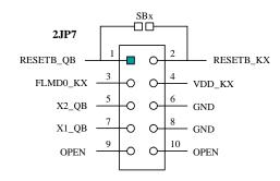
Figure 9. Micro-Board Connection to the MINICUBE
