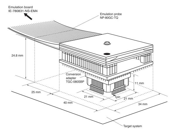
Figure B-2. Connection Condition of Target System (NP-80GC-TQ)
