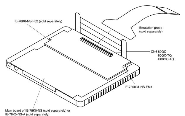
Figure 3-1. Connection of Emulation Probe
