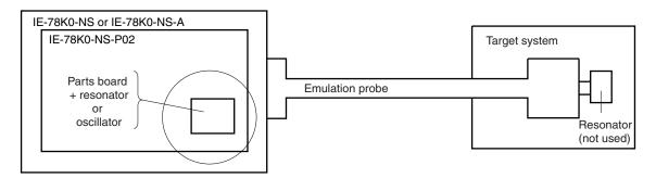
**Remark** The clock that is supplied by the IE-78K0-NS-P02's resonator or oscillator (encircled in the figure) is used.
