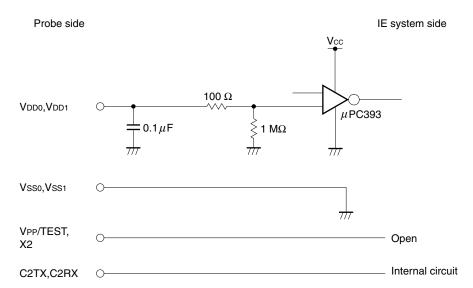
Figure 4-3. Equivalent Circuit of Emulation Circuit 3
