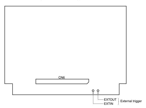
Figure 3-8. External Trigger Input Position
