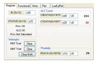
The value of internal registers is displayed on this tab. Register values cannot be set here. To set registers use the Register tab on the input side of the screen.
