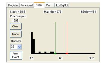
"Buckets" – allows selection of the granularity of the histogram plot. You may choose 32, 64, 128, or 256 buckets or bins to be displayed on the graph.
