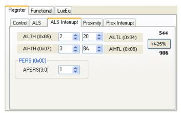
The AILT and AIHT values are 16 bit thresholds for the upper and lower trigger points. Each is set using two 8-bit registers. Another control (APERS) establishes the required persistence of the interrupt signal.
