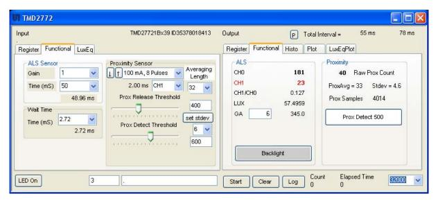
This window has inputs organized on the left, and outputs organized on the right. Values for register variables may be set using multiple techniques. The Functional tab is commonly used to quickly evaluate the device with nominal settings. The Input Register tab allows the register settings to be changed, and the Output Register tab allows registers to be viewed. Other tabs provide additional demonstration and test features for evaluation.
