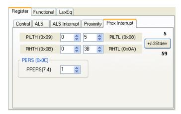
The PILT and PIHT values are 16 bit thresholds for the upper and lower trigger points. Each is set using two 8-bit registers. Another control (PPERS) establishes the required persistence of the interrupt signal.
