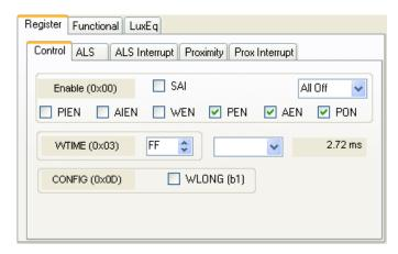
The Control sub-tab allows enabling and disabling functionality in the part and also controls the wait time multiplier (WLONG).
