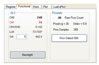
The Proximity indication shows the current reading (Raw Prox Count), a rolling average (ProxAvg), and the standard deviation of the rolling samples. The number of samples is specified on the Input Side, "Functional" tab.
