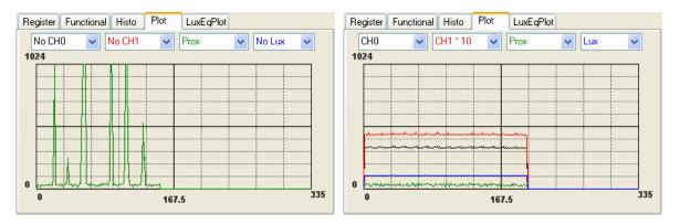
The first plot shows proximity events happening and the second graph shows all outputs for a static system. Multipliers (selected from the list boxes) may be used to scale the display accordingly. On the second plot the Ch1 photodiode is scaled by a factor of 10x relative to the other plotted signals.
