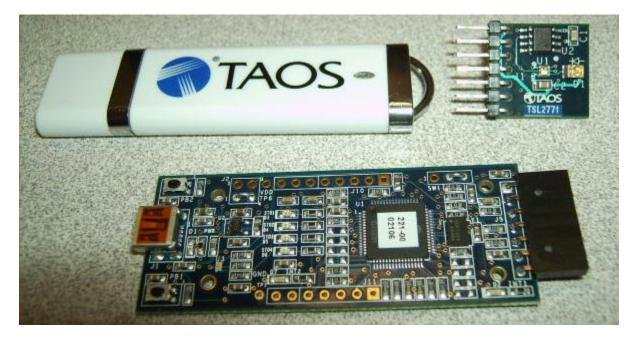
When the USB cable is connected the green LED should light up indicating that power is being received via the USB interface, and the motherboard processor is running. If the green LED does not light up, check the USB cable connections; unplug the USB cable and try again. If the green LED still does not light, check the PC for USB error messages. See the Resources section at the end of this document for additional assistance.
