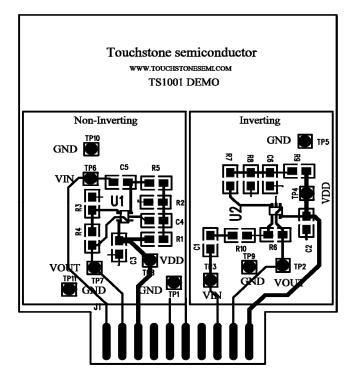
Figure 3. Top Layer Component View
