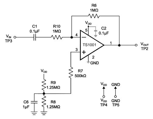
Figure 2. Inverting Configuration
