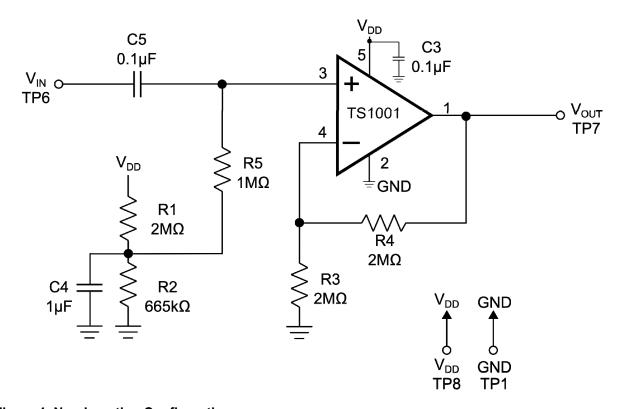
Figure 1. Non-Inverting Configuration
