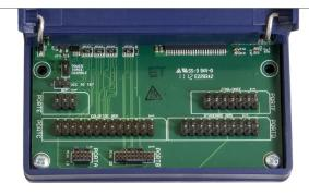
Connect the appropriate ribbon cable between the Tracelink and the target board. The Tracelink case flips open for easy access to the ribbon cable connectors. Power up the target board. A yellow LED on the Tracelink will be illuminated to indicate that it is detecting target power.
