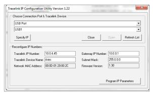
Connect the Tracelink to the PC using a USB connection. Run the ConfigureIP software utility to set up the network parameters (IP address, subnet mask, etc.). The Ethernet port will not function properly until this one-time configuration is complete. You may refer to the Tracelink User Manual for an indepth description. If the Tracelink Ethernet connection is not required, this step may be skipped.
