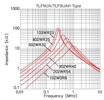
The data is reference only. Electrical characteristics vary depending on environment or measurement condition. TAIYO YUDEN reserves the right to make change to the Date at any time without notice. Before making final selection, please check product specification. 2013.11.15
