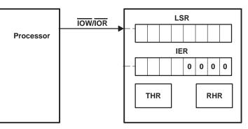
Figure 6. FIFO Polled Mode Operation
