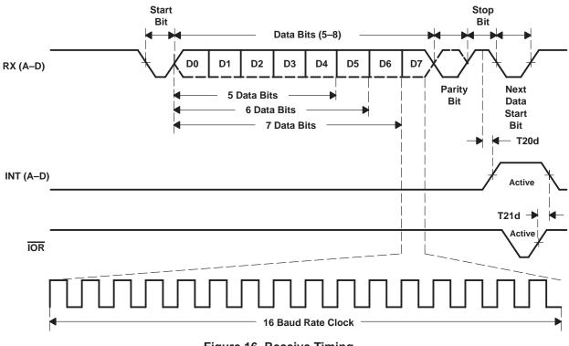
Figure 16. Receive Timing
