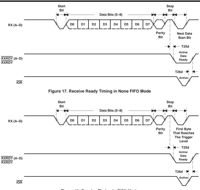
Figure 18. Receive Timing in FIFO Mode
