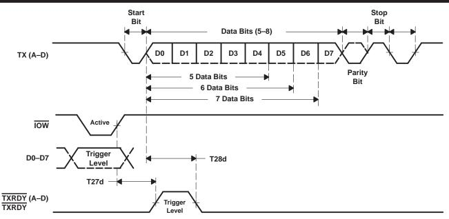
Figure 21. Transmit Ready Timing in FIFO Mode
