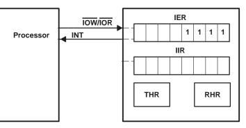
Figure 5. Interrupt Mode Operation
