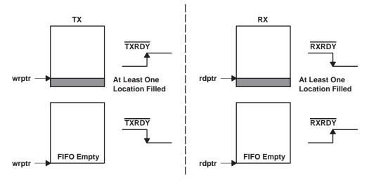
Figure 7. TXRDY and RXRDY in DMA Mode 0/FIFO Disable
