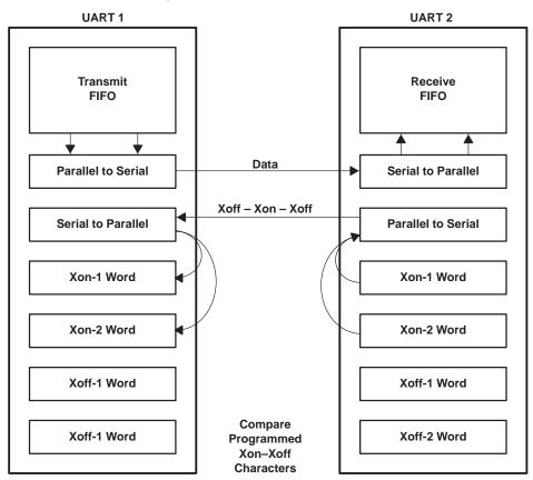
Figure 4. Software Flow Control Example
