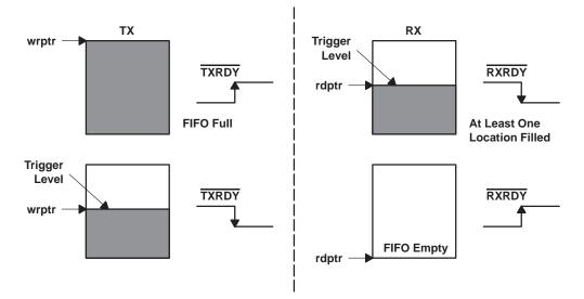
Figure 8. TXRDY and RXRDY in DMA Mode 1
