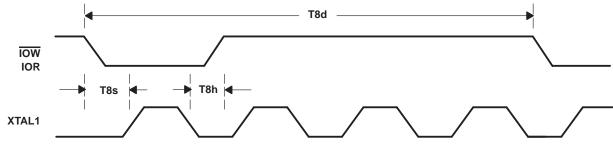
Figure 14. Alternate Read/Write Strobe Timing
