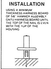
IMPORTANT: AFTER INSTALLATION, WHEN FIXTURE IS NOT IN USE, KEEP IN THE "UP" POSITION.
