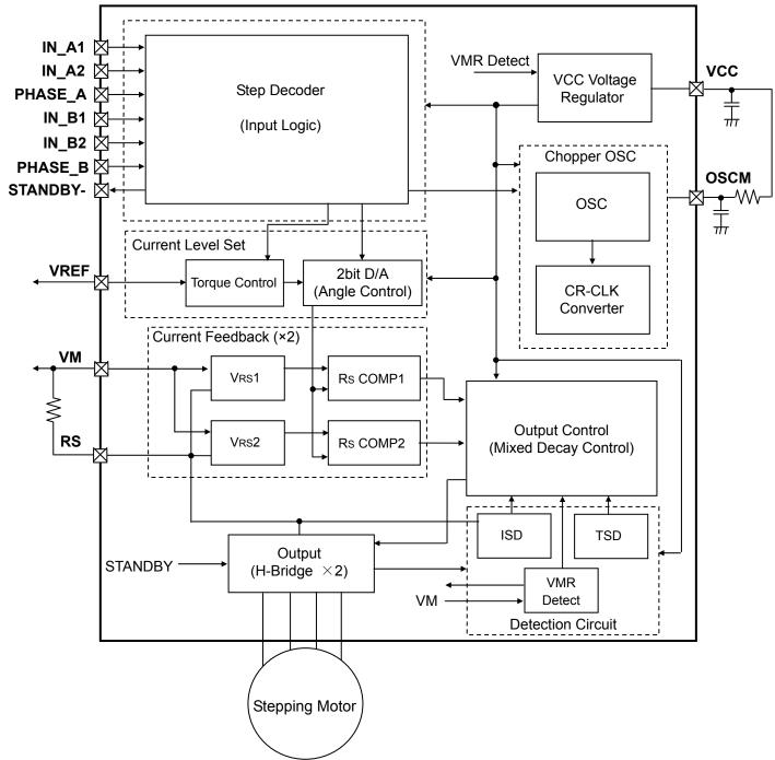
Note: All the grounding wires of the TB62213AFNG must run on the solder within the mask of the PCM. It must also be externally terminated at a single point. Also, the grounding method should be considered for efficient heat dissipation.
