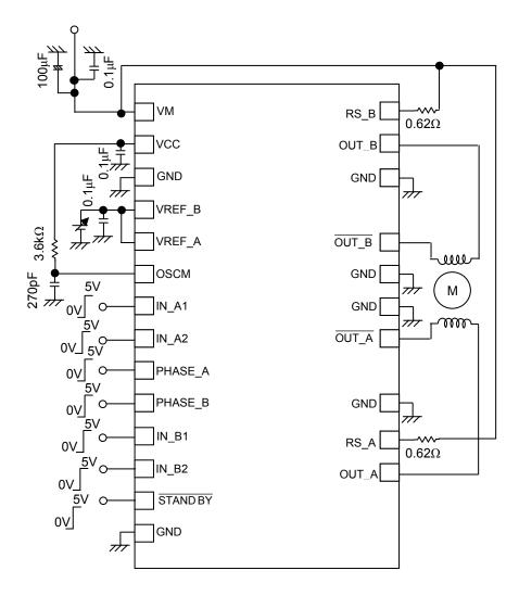
Note: I will recommend the addition of a capacitor if necessary. The GND wiring must become one point as much as possible-earth.
