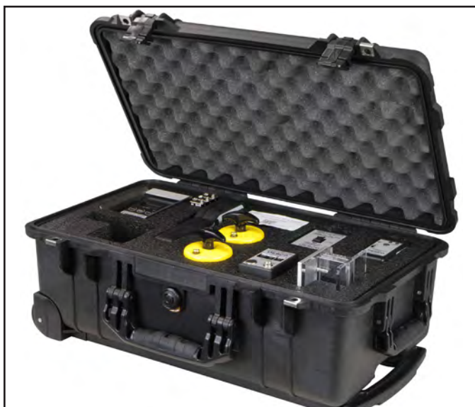
Figure 2. Desco 50569 ESD Survey Kit, Asia, 220VAC
