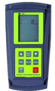
The 707 tests flue gases at home or office spaces for the presence and location of carbon monoxide leaks. This instrument fits comfortably in vour hand and operates with just the push of a button.
