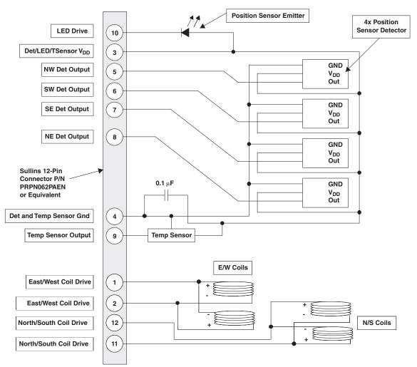
A. When a positive voltage is applied to pin #1 (a lower voltage is returned from pin #2), a beam reflected off the mirror rotates in the westerly direction. When a positive voltage is applied to pin #12 (a lower voltage is returned from pin #11), a beam reflected off the mirror rotates in the northerly direction. North and west arrows are on both sides of the package.
