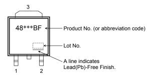
Note: The "\*\*\*" part of each product number varies according to the output voltage of the product. Be careful of static electricity when handling.
