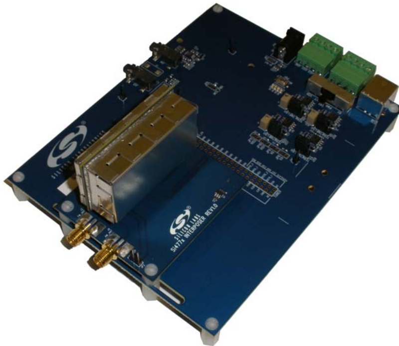
Figure 34. Si4770Module-A-EVB Module and Interposer Card
