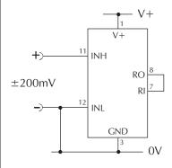
Measuring a single ended input voltage referenced to supply, i.e. the input voltage and the meter's power supply share the same 0V rail.
