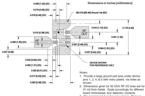
3. We recommend 1 or 2 ounce copper. Measurements for this data sheet were made on a 31 mil thick Getek with 1 ounce copper on both sides.
