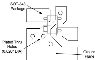
Use multiple plated-thru via holes located close to the package pins to ensure a good RF ground connection to a continuous groundplane on the backside of the board.
