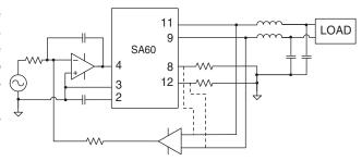
one translates the differential output voltage to a single feedback voltage. Dashed line connections and a higher gain difference amplifier would be used for current control. The error amplifier integrates the difference between the input and feedback voltages to close the loop.
