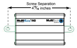
2. To attach the mounting bracket to the modem, slide the brackets through the slot on the back of the chassis.
