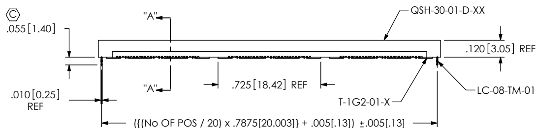
FIG 1 -LC: LOCKING CLIP OPTION SHOWN
