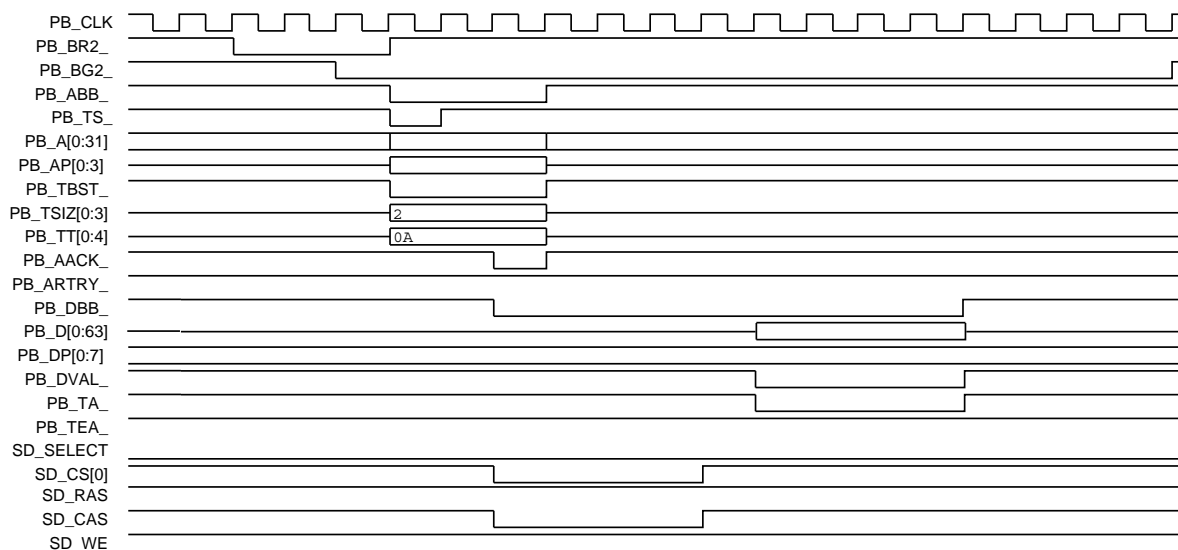
Figure 23: Burst Read with Logical Bank Open at the Required Address
