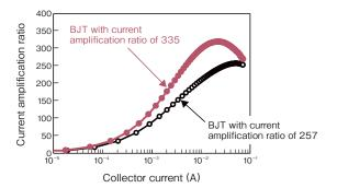
Fig. 1 Current amplification ratio over 200 Current amplification ratio for BJT prototyped by Kyoto University. (Based on material courtesy Kyoto University)
