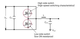
Fig. 1 Power device configuration in DC-DC converter High-side switch and low-side switch are used in DC-DC converter circuits.
