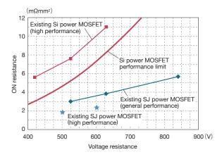
Approaching the performance limits of Si power devices The introduction of super-junction architecture has made it possible to exceed the performance limits of standard power MOSFETs, but it will be difficult to improve the ON resistance much more. (Courtesy Infineon Technologies)
