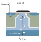
Super-Junction power MOSFET structure Compared to the standard power MOSFET, the p layer is significantly deeper.
