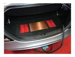
Fig. 2 Power amplifier in trunk of Mercedes-Benz SLR McLaren Roadster The use of SiC SBDs stabilized power amp operation, thereby improving audio quality.
