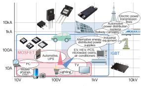
Fig. 1 Expanding range of application for power devices
