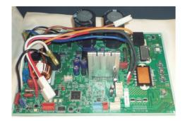
Fig. 2 Inverter module The air conditioner inverter board. The red dashed circle is the inverter module, with SiC SBDs mounted.
