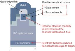
Cell pitch tightened up from standard 6µm to 4µm
