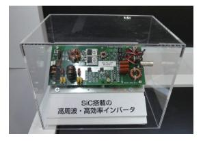
Fig. 3 Wireless power supply system inverter The transmitter inverter circuit uses SiC trench-type MOSFETs.
