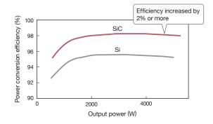
Fig. 2 98% conversion efficiency Conversion efficiency was improved to 98%, up 2%, through the use of SiC power devices. (Based on material courtesy Mitsubishi Electric.)
