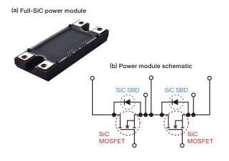
The volume-production full-SiC module is currently only available in one specification: rated voltage 1200V, rated current 100A. Although the rated current is only 100A, high-speed switching and lower loss means it can be used to replace Si IGBT modules for 200A to 400A applications. If used to replace a 400A class Si IGBT, says ROHM, it would roughly halve needed volume.
