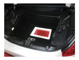
Fig. 1 Power amplifier in Peugeot 308CC trunk The SiC SBDs in the power amp were jointly developed by Bewith Enterprise and New Japan Radio.
