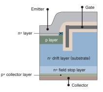
IGBT device structure The input section is MOS, and the output bipolar. (Courtesy Infineon Technologies)
