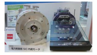
Fig. 3 Driving system developed by ROHM and Yaskawa Electric Motor integrated with winding selector, inverter, and controller (including gate driver IC and microcontroller).
