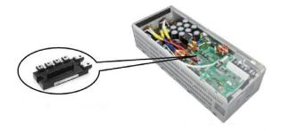
Fig. 1 Power conditioner for photovoltaic systems Mitsubishi Electric has prototyped a power conditioner for photovoltaic systems using a full-SiC power module. (Courtesy Mitsubishi Electric.)
