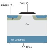
Representative power MOSFET structure The diagram shows a standard structure, combining a low ON resistance with high-speed switching characteristics.
