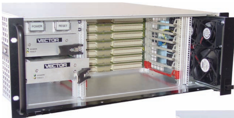
Model 761: 7 Slot VME64x-Hinged Smoked Glass Door (open)
