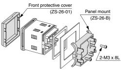
Tighten screws 1/4 to 1/2 turn after the heads are flush with the panel.
