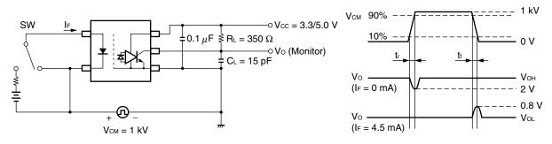
**Remark** C<sub>1</sub> includes probe and stray wiring capacitance.
