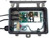
Reattach the protective covering over the PC board and terminal blocks and re-close the lid. Ensure that the four captive screws are fully tightened before operation can commence.
