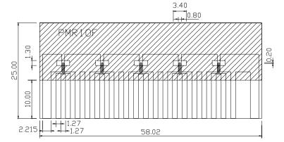
NOTE) \*1 The shaded area shows the solder resist treatment.
