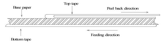
4.2 Base tape should not adhere to top tape when top tape is peeled back, and peel back direction is as follows.
