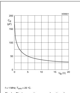
Fig.4 Diode capacitance as a function of reverse
