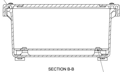
(4) EACH #10-32 BRASS INSERTS AND PLATED CARBON STEEL SCREWS
