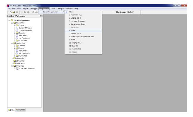
Wait while MPLAB is downloading operation system, and after Pic-Kit3 is connected – check in menu Programmer – Settings – Power – there is option – Power target circuit from PicKit3 – this option should be forbidden, you could not select it. Now it is safe to connect the programmer to your target board trough an ISCP cable. The PIC-WEB should be connected to the power supply.
