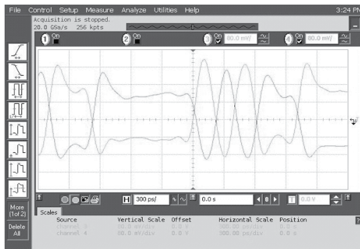
Data Waveforms, 2.5Gbps (left) & 5.0Gbps (right)
