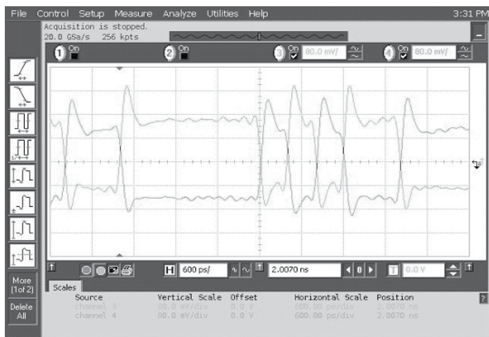
Data Waveforms, 2.5Gbps (left) & 5.0Gbps (right)
