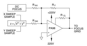
perhaps automatic focusing circuitry might be used to generate this potential. The dynamic correction is generated from the sweep voltages by calculating the distance of the beam from the center of the display.
