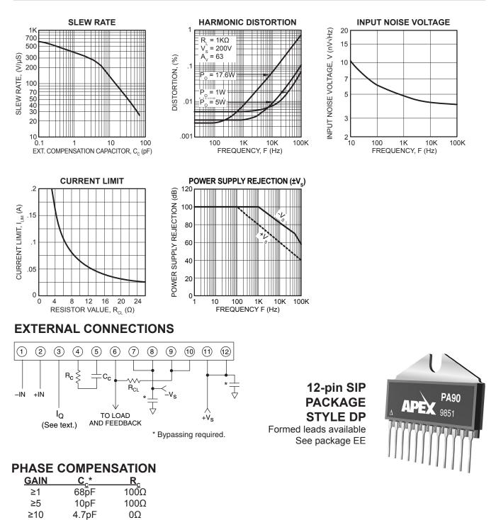
$^{*}\mathrm{C}_{_{\mathrm{C}}}$  To be rated for the full supply voltage +V  $_{_{\mathrm{S}}}$  to –V  $_{_{\mathrm{S}}}$ . Use NPO ceramic (COG) type.
