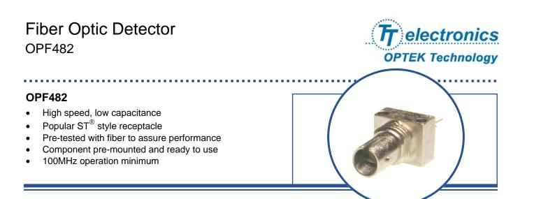
The OPF482 is a low noise silicon PIN photodiode mounted in a low cost package for fiber optic applications. It offers fast response at moderate bias and is compatible with LED and laser diode sources in the 800-1000 nm wavelength region. Low capacitance improves signal to noise performance in typical short haul LAN applications.
