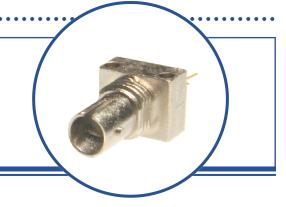
The OPF432 is a low noise silicon PIN photodiode mounted in a low cost package for fiber optic applications. It offers fast response at moderate bias and is compatible with LED and laser diode sources in the 800-1000 nm wavelength region. Low capacitance improves signal to noise performance in typical short haul LAN applications.
