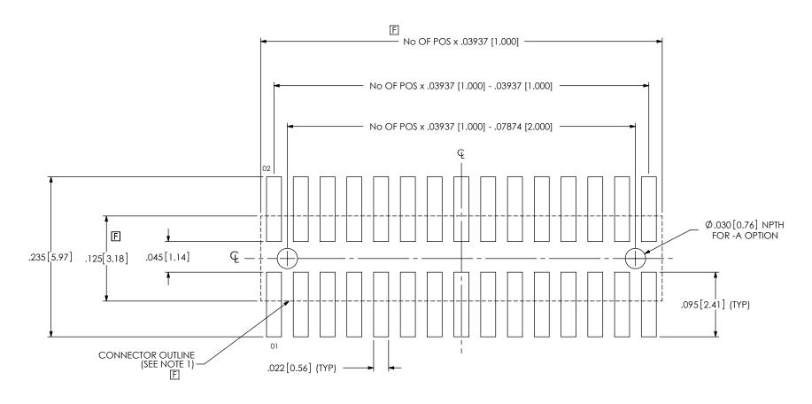
FIG 1 MW-15-03-X-D-XXX-XXX SHOWN ALL DIMENSIONS ARE SYMMETRIC ABOUT THE CENTERLINE.
