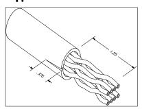
Remove 1.25" (31.8 mm) of cable jacket. Slit both sides of jacket back .375" (9.5 mm). The slits should be located where the two outer pairs exit jacket. Separate the pairs.
