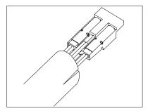
Turn assembly over and insert center pair into loadbar.
