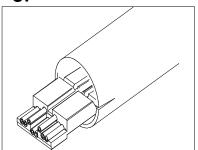
Ensure that all conductors are flat and straight in loadbar area. Trim all conductors flush with edge of loadbar.
