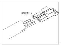
Insert outer pairs of conductors into loadbar as shown.
