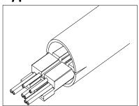
Push loadbar back onto cable until the edge of jacket is even with the notch in the loadbar. Pull any slack out of the conductors. Twist should be as close to loadbar as possible for best performance
