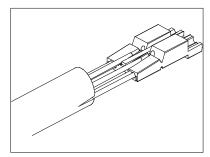
Turn assembly back. Trim the last pair slightly to make loading easier and insert into loadbar.
