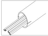
Straighten conductors and align per diagram Only untwist enough conductors to allow insertion into loadbar.
