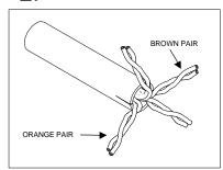
Arrange pairs according to appropriate wiring diagram (see back of sheet). If pairs need to be crossed, keep twisted and cross inside jacket.
