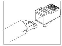
Insert loadbar into the housing and terminate.
