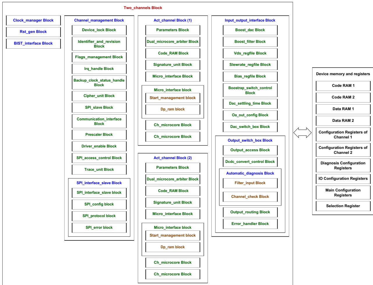
Figure 22. Device Logic Block Hierarchic Overview
