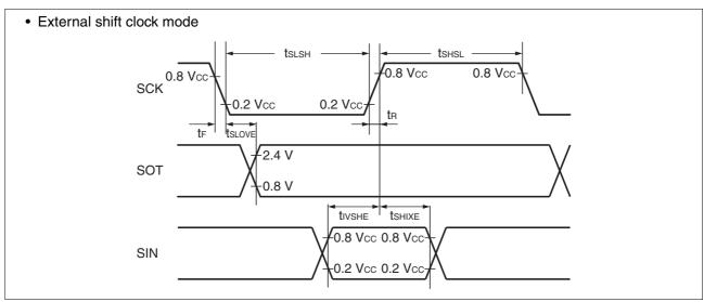
Sampling is executed at the falling edge of the sampling  $clock^{*1}$ , and serial clock delay is disabled  $clock^{*2}$ . (ESCR register: SCES bit = 1, ECCR register: SCDE bit = 0)
