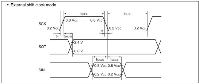
Sampling is executed at the rising edge of the sampling  $clock^{*1}$ , and serial clock delay is enabled\*2. (ESCR register: SCES bit = 0, ECCR register: SCDE bit = 1)
