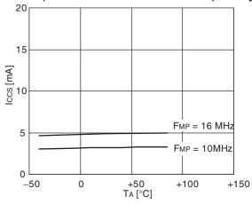
$\label{eq:ccl} \begin{array}{c} I_{CCL}-T_{A} \\ Vcc=5.5~V~F_{\text{MPL}}=16~kHz~(divided~by~2) \\ Subclock~mode~with~the~external~clock~operating \end{array}$
