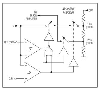
Figure 5. Dual-Mode Feedback Decoder
