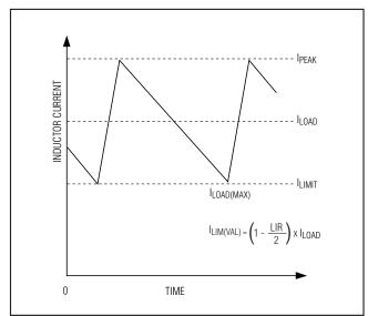
Figure 4. Valley Current-Limit Threshold
