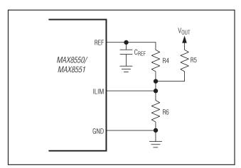
Figure 7. Foldback Current Limit
