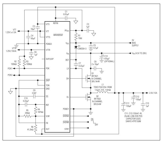
Figure 8. Typical Applications Circuit
