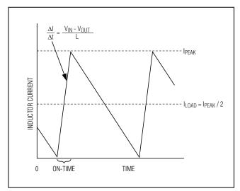
Figure 2. Pulse-Skipping/Discontinuous Crossover Point
