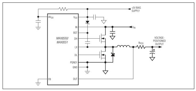
Figure 9. Voltage-Positioned Output
