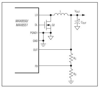
Figure 6. Setting VOLIT with a Resistive Voltage-Divider
