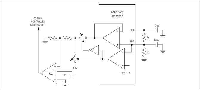
Figure 3. Adjustable Current-Limit Threshold
