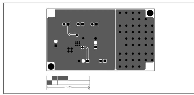
Figure 4. MAX16803EVKIT+BJT PCB Layout—Solder Side
