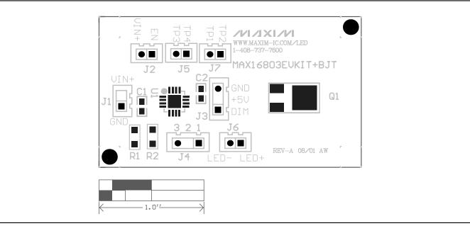
Figure 2. MAX16803EVKIT+BJT Component Placement Guide—Component Side
