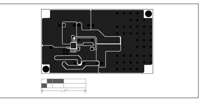
Figure 3. MAX16803EVKIT+BJT PCB Layout—Component Side
