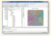
Easy graphical assignment of signals to pins and a graphical representation of SSO noise analysis.
