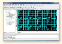
A detailed, read-only view of the physical routing of paths for a more detailed understanding of timing issues.
