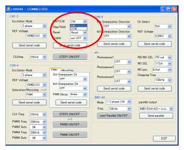
Also, when the stepping motor is driven, the frequency of the reference clock signal "STEP1" is set.
