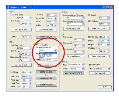
Also, "Frequency" and "PWMduty" of the PWM signal are set to the pins "PWM3 STEP2" and "PWM4".
