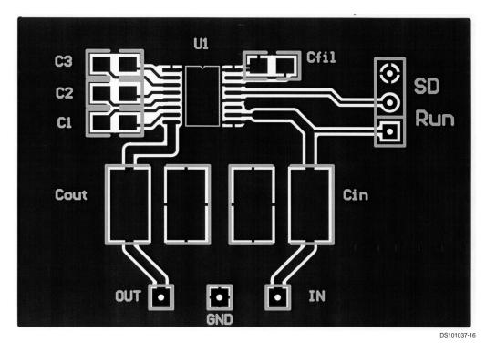
FIGURE 4. Typical Layout, Top View (magnification 2.8X)
