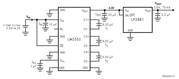
FIGURE 3. Low Output Noise and Ripple Buck/Boost Regulator
