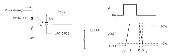
\*5. Reference value : min = 2.6V and typ = 2.8V when  $V_{\mbox{CC}}$  = 2.9V
