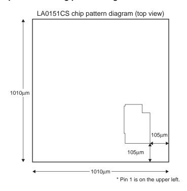
LA0151CS photo-receiving pattern enlarged diagram (effective area)
