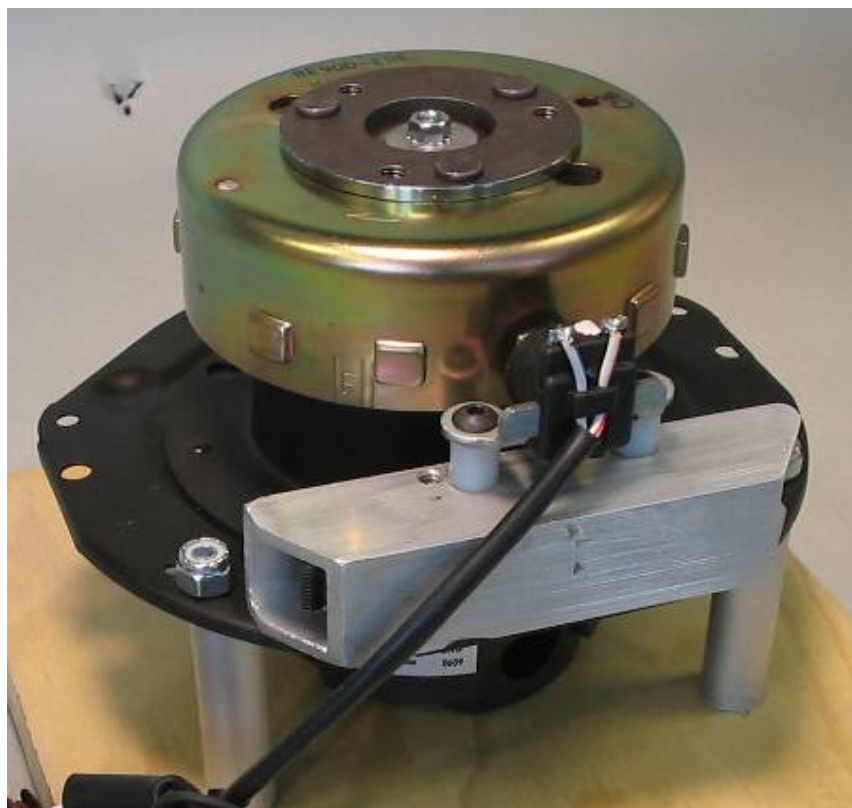
Figure 7. Spin Bench Example for Creating a Physical Simulated Engine Position Signal
