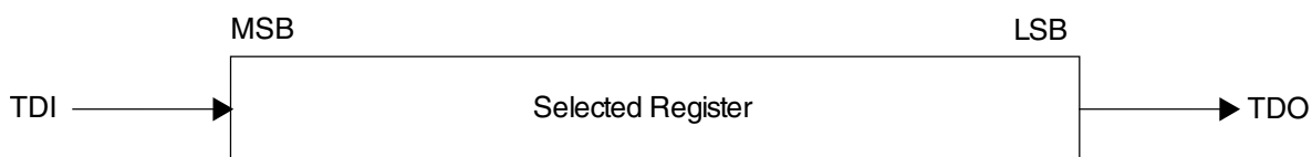
Figure 53-3. Shifting data through a register
