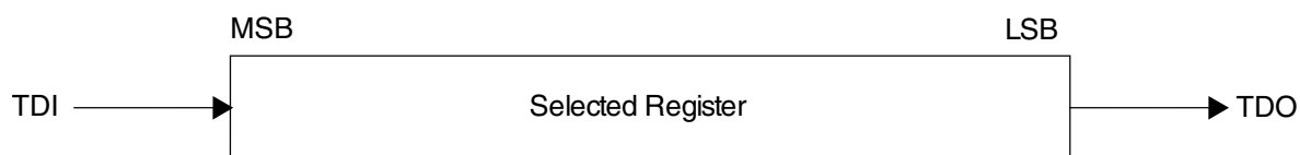
Figure 54-3. Shifting data through a register
